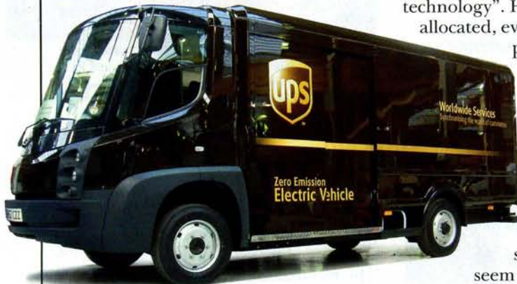
Modec produce electric vehicles of this size with over 100 mile range carrying 2 tonne payload from a single overnight charge. www.modec.co.uk
