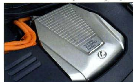
Lexus hybrid GS450h. The electric motor works in harmony with the 3.5-litre V6 engine to produce power normally associated with a V8 and the economy of a 2.0-litre 4-cylinder.
