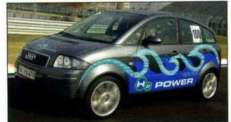
The 2004 Audi A2-H2 concept car emits nothing but pure water vapour, yet offers performance similar to a petrol-powered A2.
