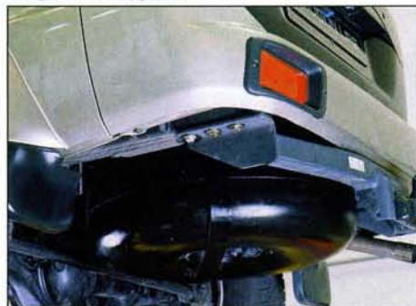
No loss of luggage space for this Shogun as the tank is mounted under the rear floor!
